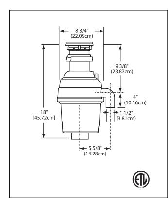
MOTOR HORSEPOWER 3/4 HP
